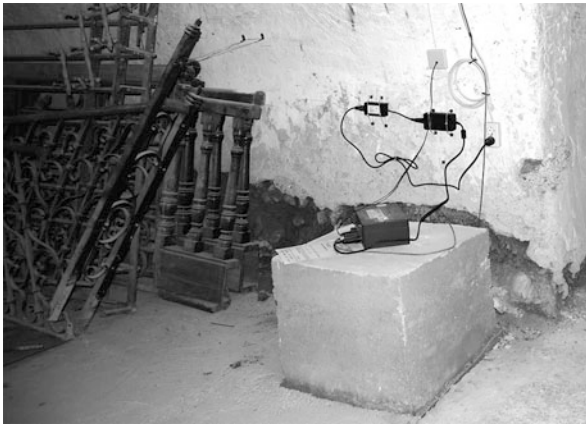
Fig. 5.3 The accelerometric station in the basement of the old jailhouse, Lorca
