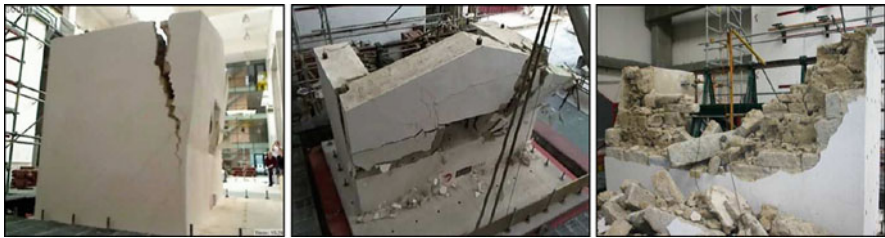
Fig. 8.23 Failure mode of subassembly (Costa et al. 2012a)
