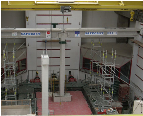
Fig. 4.31 Shake table test of the beam-to-column dowel connection at LNEC
