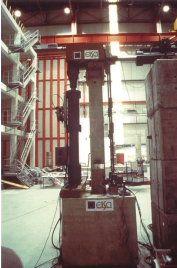
Fig. 4.16 ASSOBTION tests on precast columns with pocket foundation performed at ELSA
